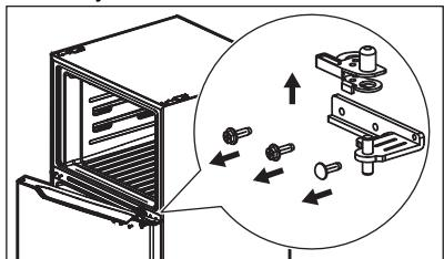
4. Unscrew and remove the bottom hinge.
