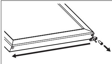
9. Place the bottom left corner of the door onto the lower hinge, then install top hinge to the cabinet. Make sure the door is level and it seals properly against the cabinet. Securely fasten
