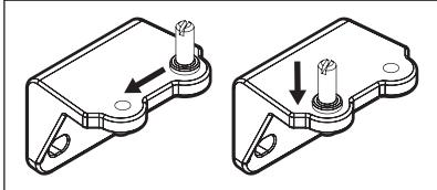
7. On the bottom edge of the door, transfer the door stop bracket and bushing to the holes on the opposite side.
