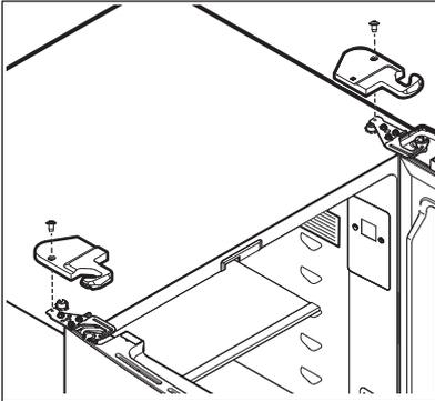
2. Disconnect electrical harness running from door to hinge cover.
