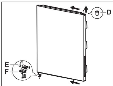
7. Remove the central hinge and hinge shaft with slotted screwdriver.
