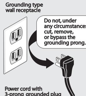
Avoid fire hazard or electrical shock. Do not use an adaptor plug or extension cord or remove grounding prong from electrical power cord. Failure to follow this warning can cause serious injury, fire or death.
