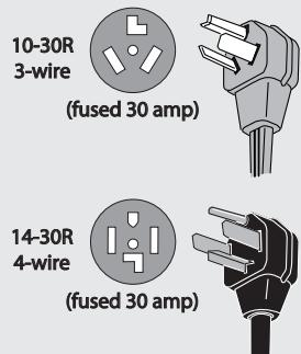
UL-approved service cord must be installed on electric dryers (not provided with unit except those manufactured for sale in Canada).
