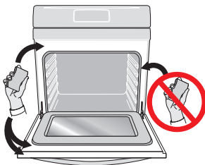
Figure 24: Clean around the oven door gasket
