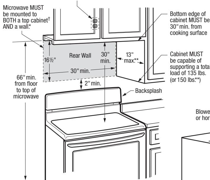
†When installing beneath smooth, flat cabinets, refer to cabinet template for detailed power cord clearance instructions
