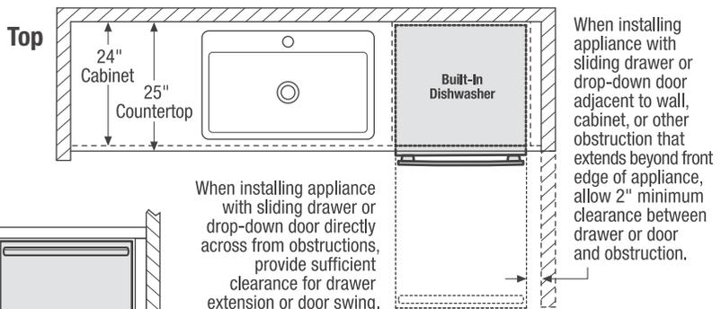
Use these dimensions and clearance instructions for planning purposes only. For detailed installation instructions, refer to installation guide, packed with product, or on the web at frigidaire.com.
