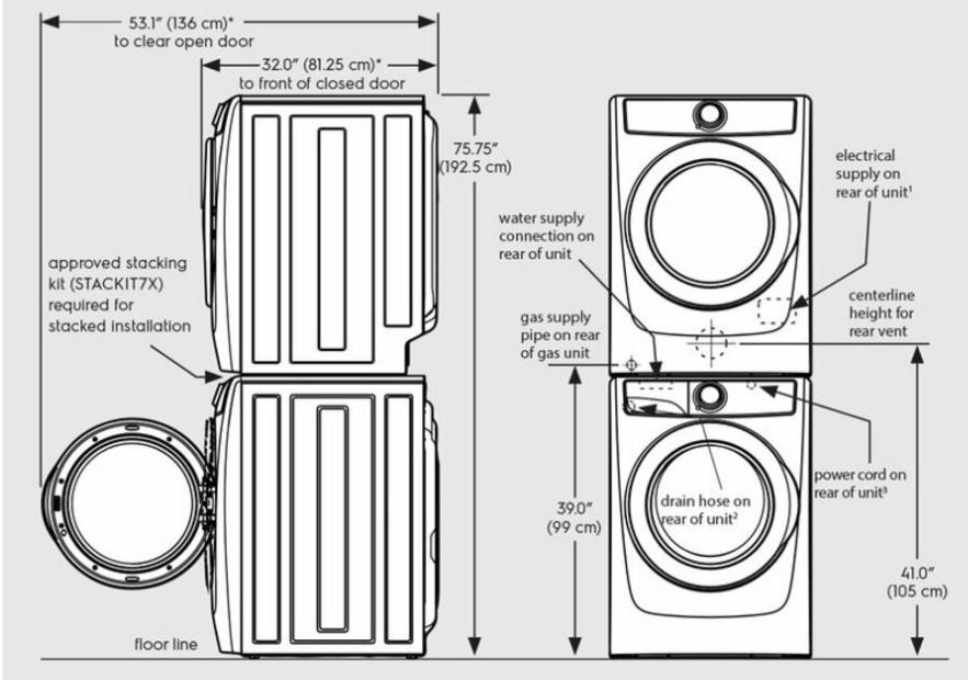
\* Connection of water inlet hose on steam dryer adds 3/4 in. (2 cm) to installation depth.
