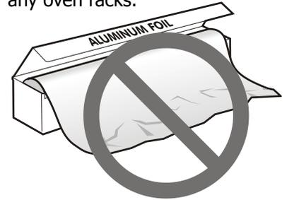
During self-clean the oven temperature can become hot enough to melt aluminum cooking utensils or aluminum foil if left in the oven. This could result in damage to the oven interior porcelain finish.
