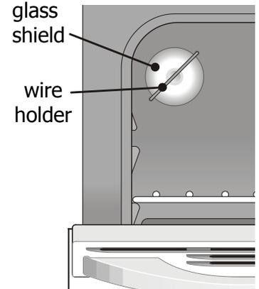
The glass shield should always be in place to protect and shield the oven interior light whenever using the oven.
