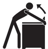
To check if the anti-tip bracket is installed properly, use both arms to grasp the rear edge of the appliance back. Carefully attempt to tilt appliance forward. When properly installed, the appliance should not tilt forward.
