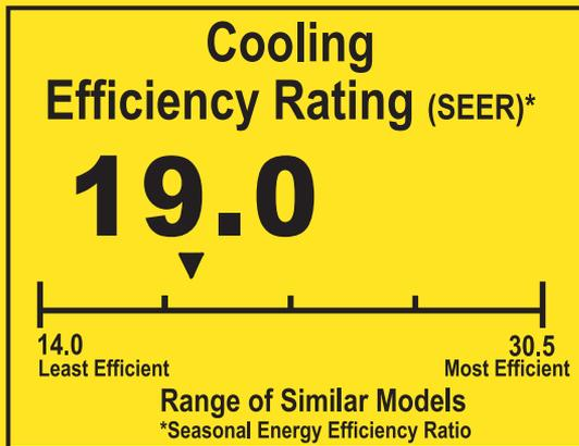
▼▼ This system's efficiency rating depends on the coil your contractor installs with this unit. The heating efficiency rating varies slightly in different geographic regions. Ask your contractor for details.
