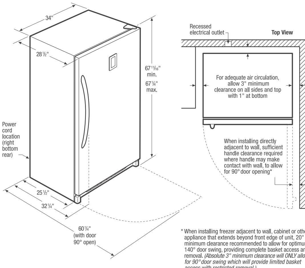
\* When installing freezer adjacent to wall, cabinet or other appliance that extends beyond front edge of unit, 20" minimum clearance recommended to allow for optimum 140° door swing, providing complete basket access and removal. (Absolute 3" minimum clearance will ONLY allow for 90° door swing which will provide limited basket access with restricted removal.)
