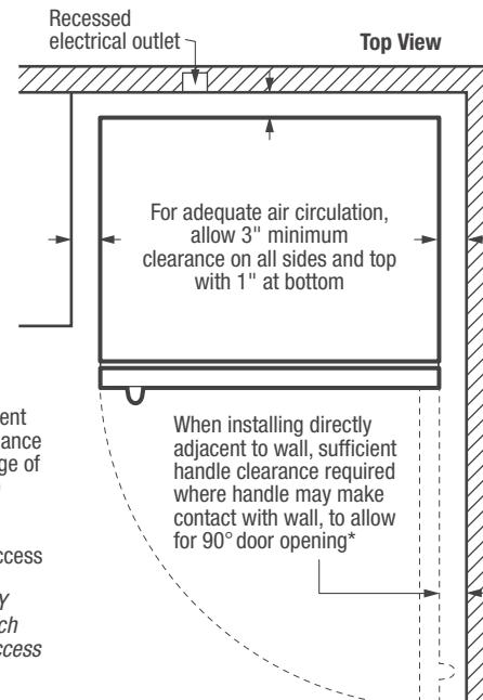
\* When installing freezer adjacent to wall, cabinet or other appliance that extends beyond front edge of unit, 20" minimum clearance recommended to allow for optimum 140° door swing, providing complete basket access and removal. (Absolute 3" minimum clearance will ONLY allow for 90° door swing which will provide limited basket access with restricted removal.)
